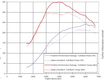
The improved performance is produced through a carefully developed combination of matched induction, exhaust and engine management modifications.
